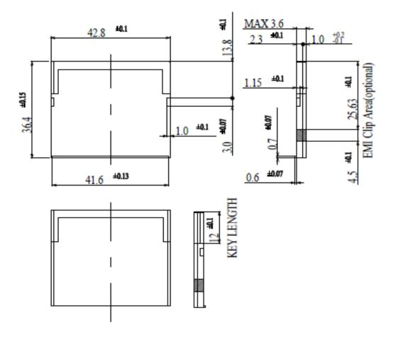
Figure 2-1. Type I CFast Card Dimensions
