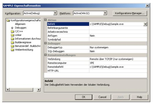
figure 10 - Remote Debugging Setup
