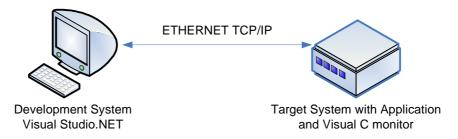
figure 9 - Remote Application Debugging
