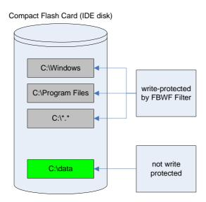
figure 1 - Compact Flash FBWF setup
